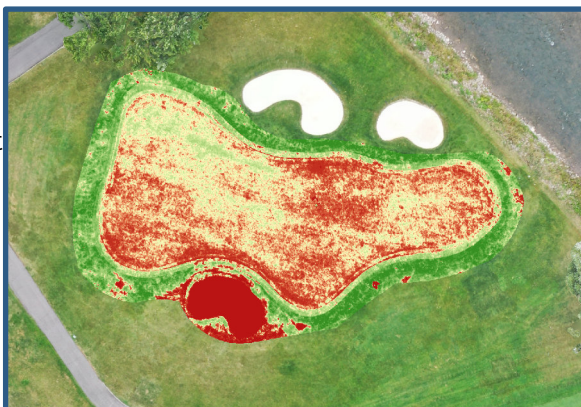
Figure 5: A closer look at a green using NDVI shows areas where there has been more foot traffic due to pin placements.
