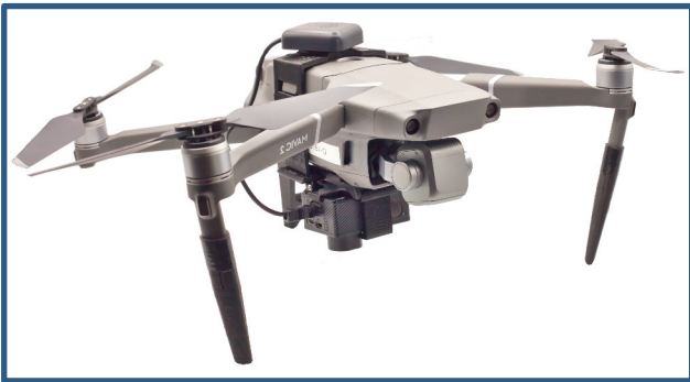
Figure 2: A drone that can be used to conduct the surveys of the course to create NDVI images.
