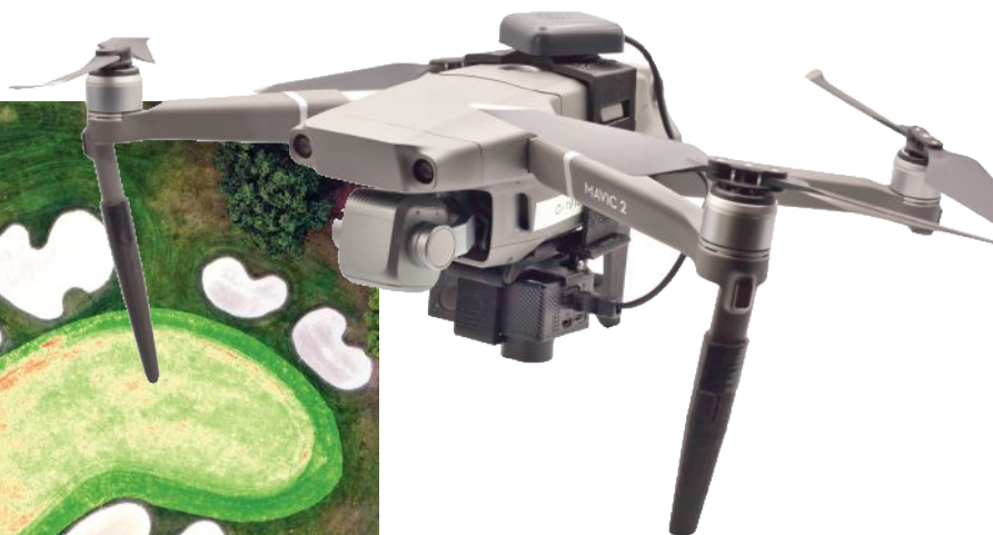
Figure 5: A drone that can be used to conduct the surveys of the course to create NDVI images.
